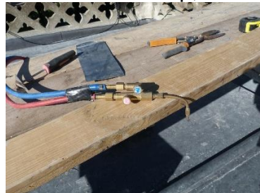
Tools for cutting and welding
